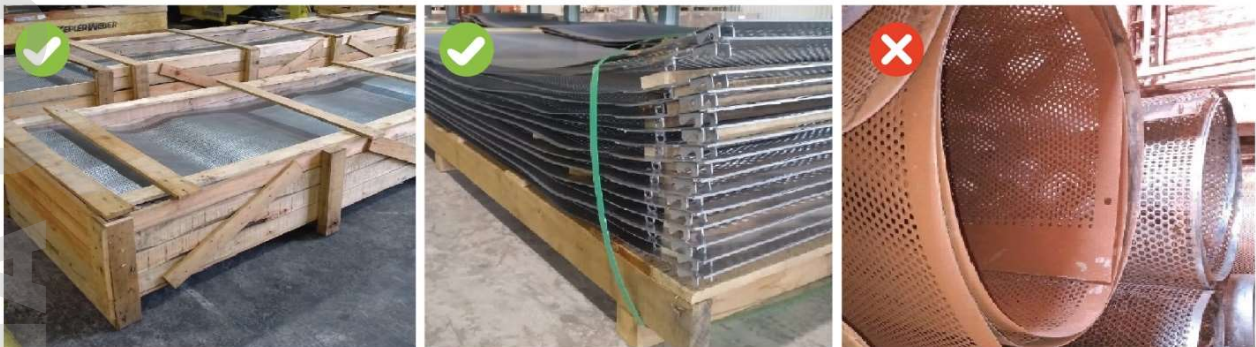
Figure 21 – Storage of MLR Cleaning machine sieves..
